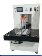
Applied to automatic edge cutting, single folding, double folding, edge ironing, shaping of pouch cell.
