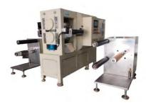
Suitable for thinning and increasing density of lithium battery electrodes, in order to achieve the designed/predetermined volumetric energy density and battery performance of lithium batteries produced by rolled electrodes.
